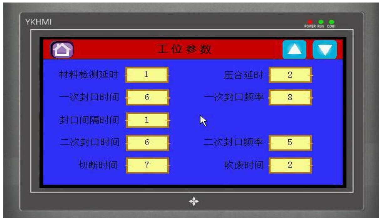
5.2.2 点击各数字框
