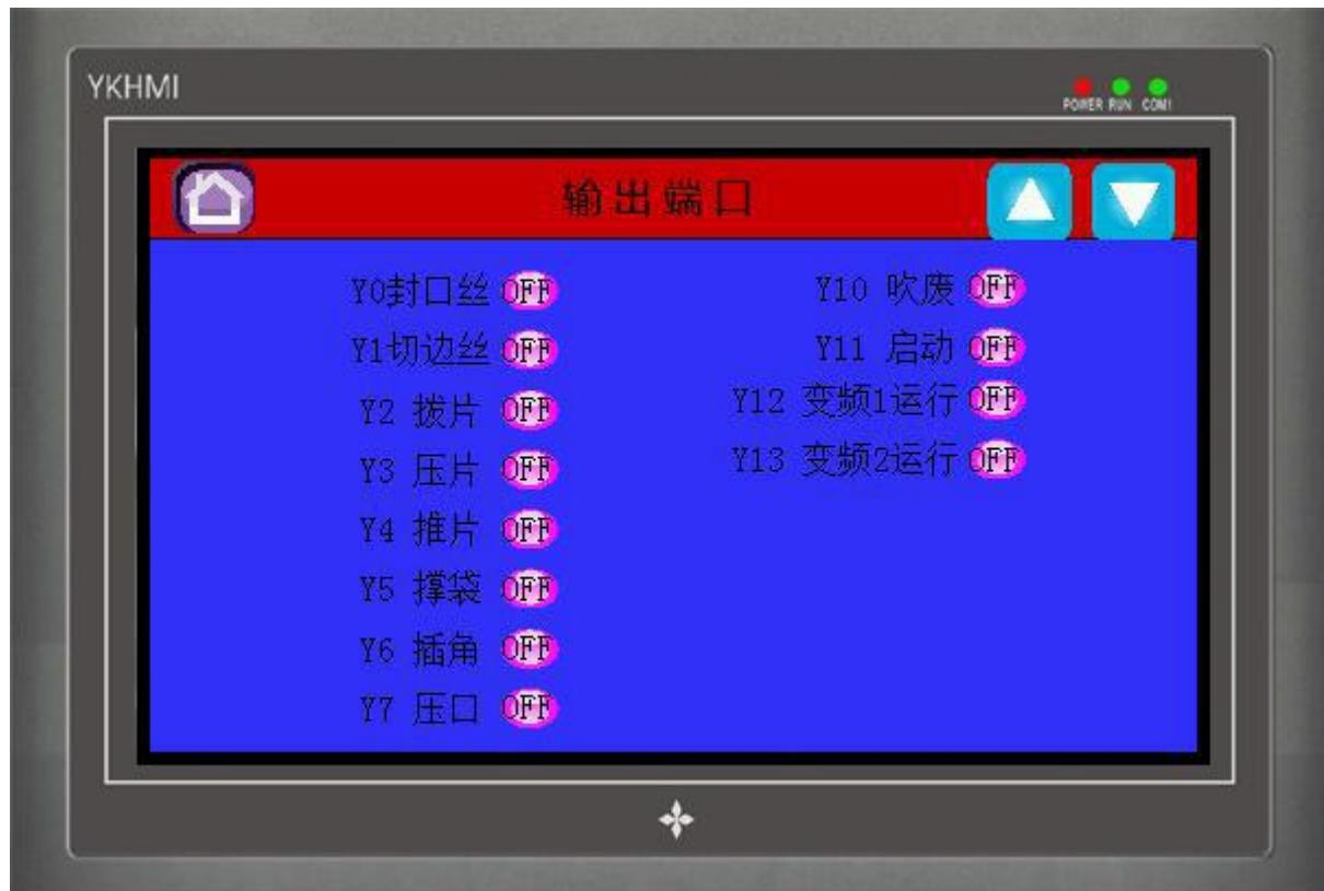
The packaging machine controls each solenoid valve by PLC, and then each cylinder is driven by a solenoid valve. This screen is used to judge whether or not each solenoid valve operates in the order set by the program.
